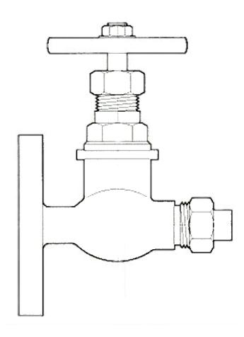
This fitting is suitable for pressure gauge take-off connections etc.
